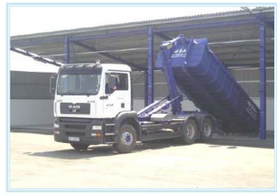
Container-loading vehicle for bulky waste
