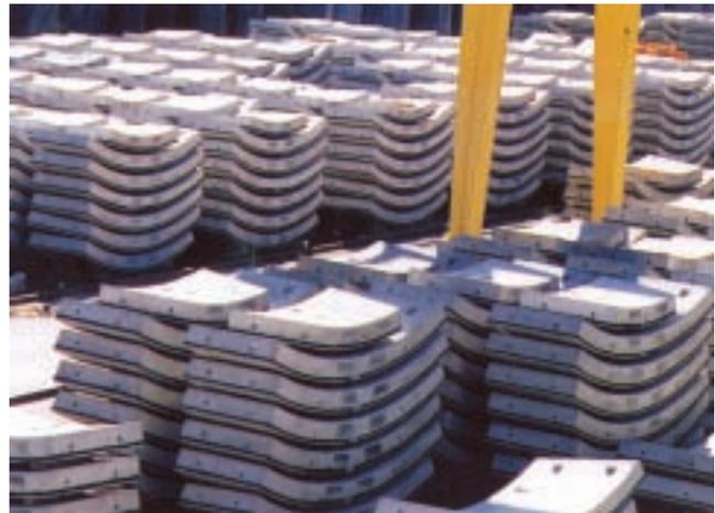
Prefabricated tunnel lining segments
