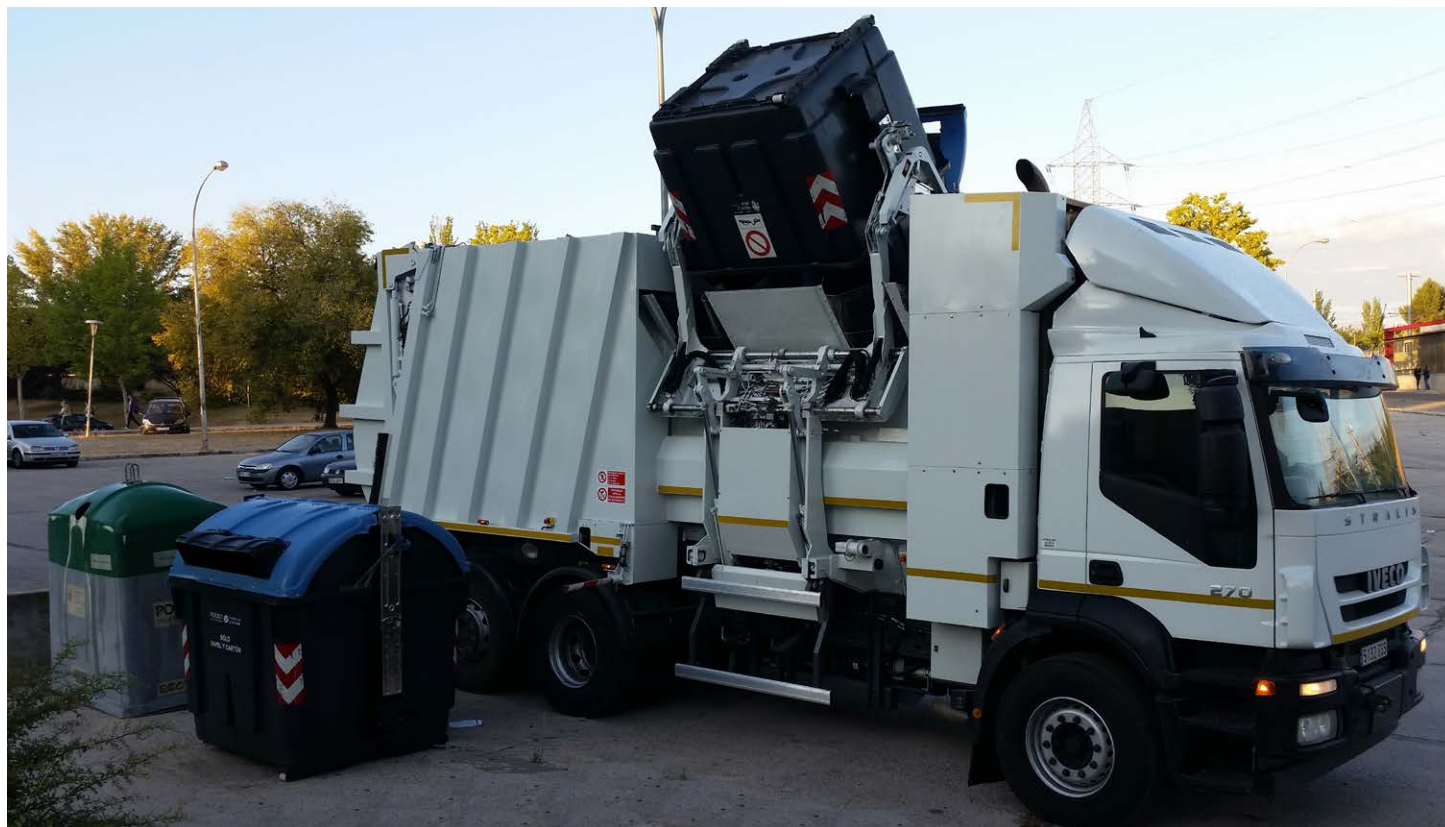
Ultra-capacitor vehicle for MSW.
