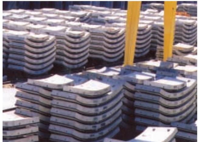
Prefabricated tunnel lining segments
