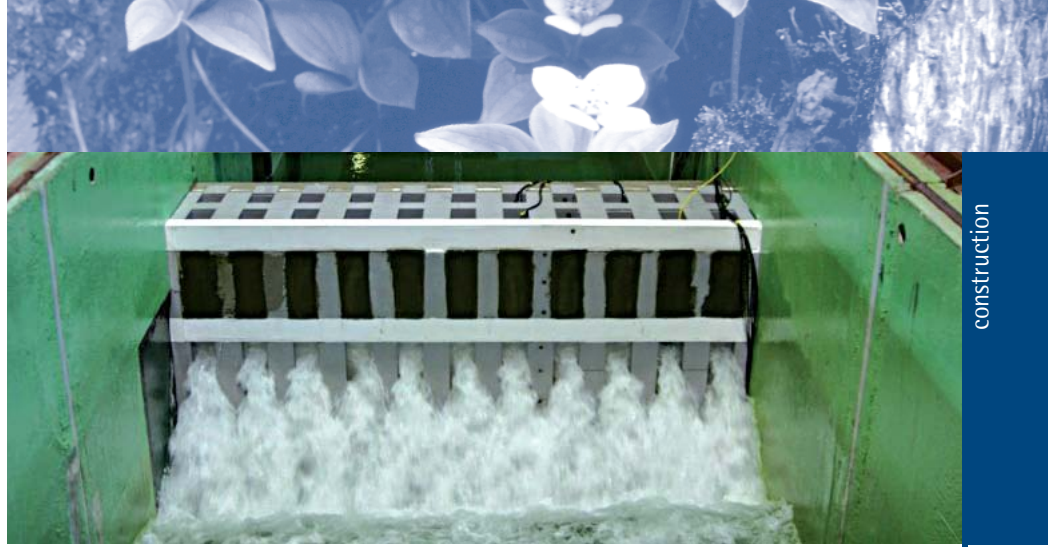
Low reflection caissons for wharves and seawalls
