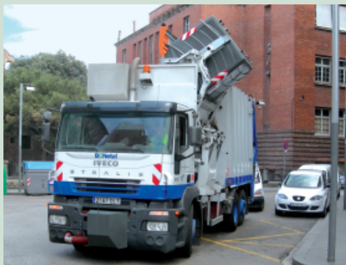
Urban solid waste collection. Side-loading collection vehicles, Barcelona
