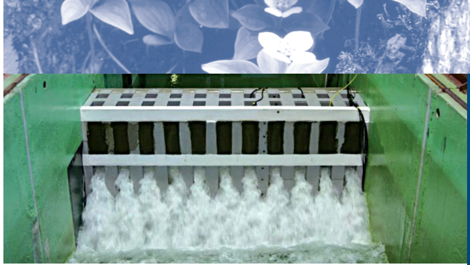
Low reflection caissons for wharves and seawalls
