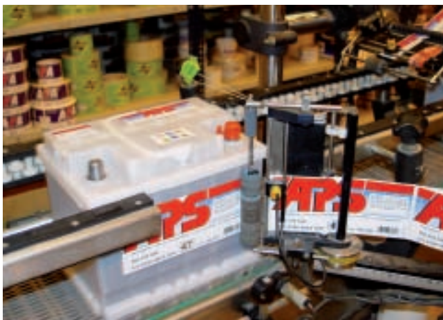
Logistics. Automatic battery labelling
