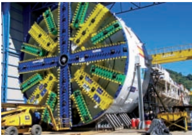
"Tizona", one of FCC's tunnel boring machines
