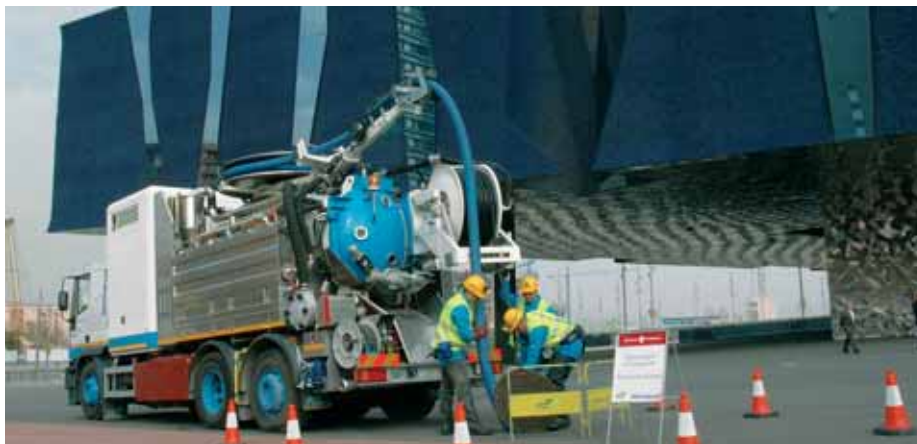
Vehicles combining vacuum pumps and water jets to clean sewer systems
