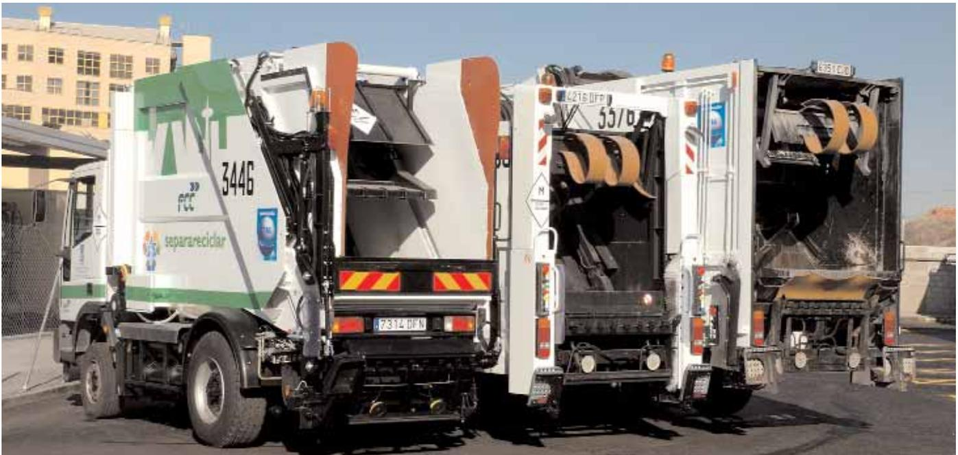
The reduced size vehicle, which is 1.8 wide, makes it possible for this gas-powered vehicle to get into the very tight spots which are commonly found in the centres of Spanish cities. This vehicle, which is about as wide as many private cars, loads and compacts almost 4 tm of trash, which is the equivalent of collecting the waste generated by almost 4,000 residents on each trip.
