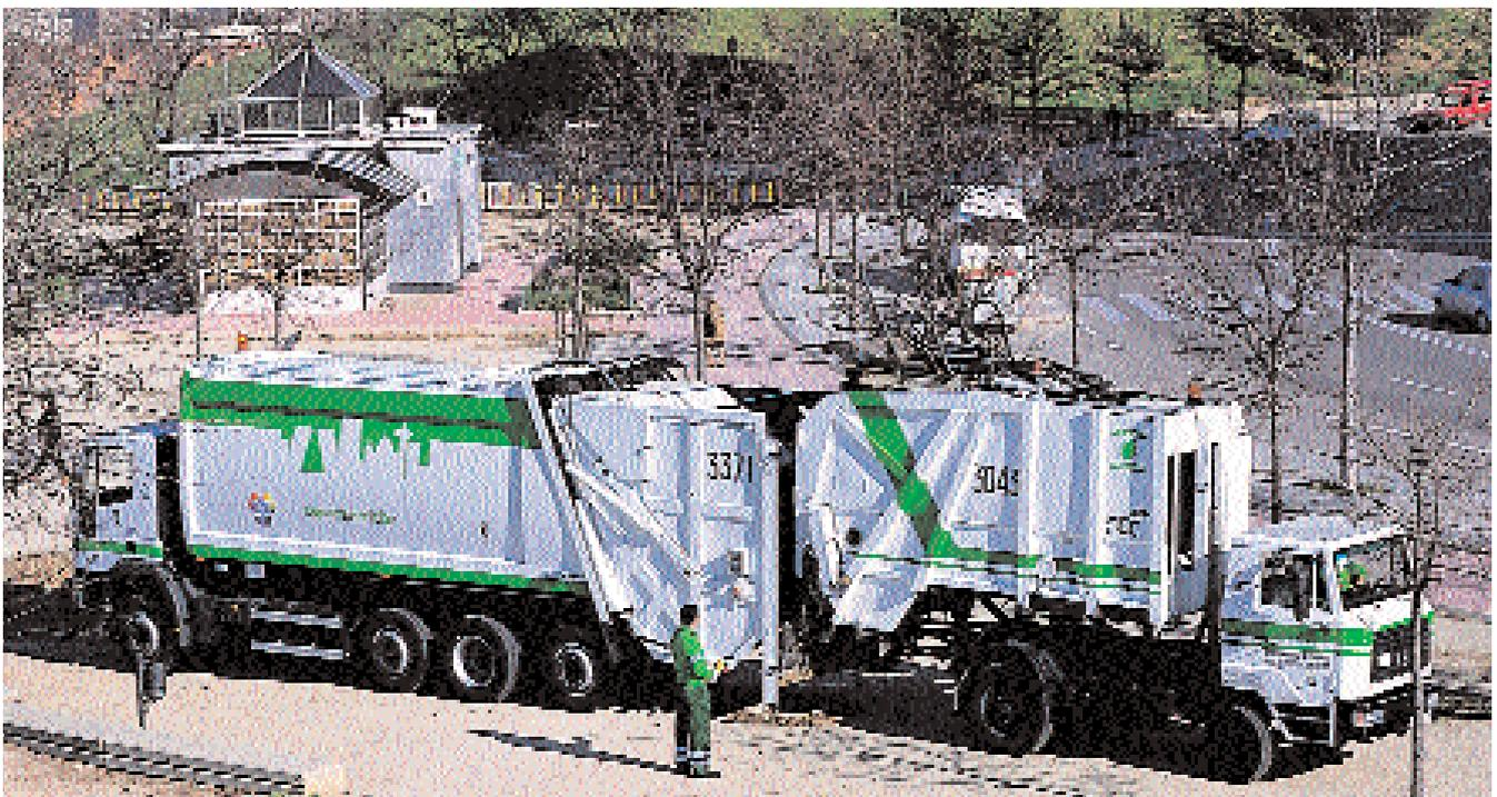
axles is very short in order to obtain a minimum turning radius, 27 m<sup>3</sup> of body volume and a maximum length of 10.5 m.
