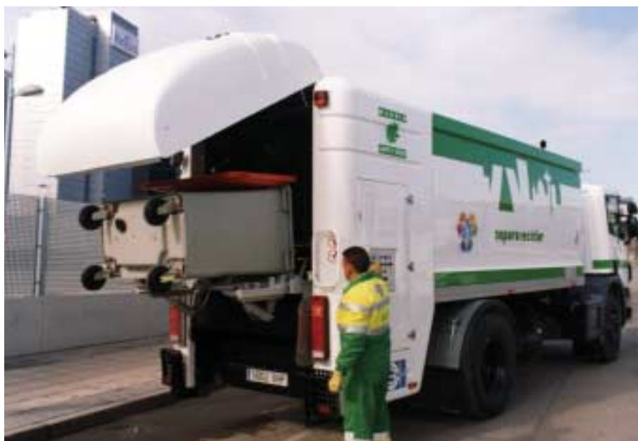
Hermetic containing cleaning with recycle water. Madrid
