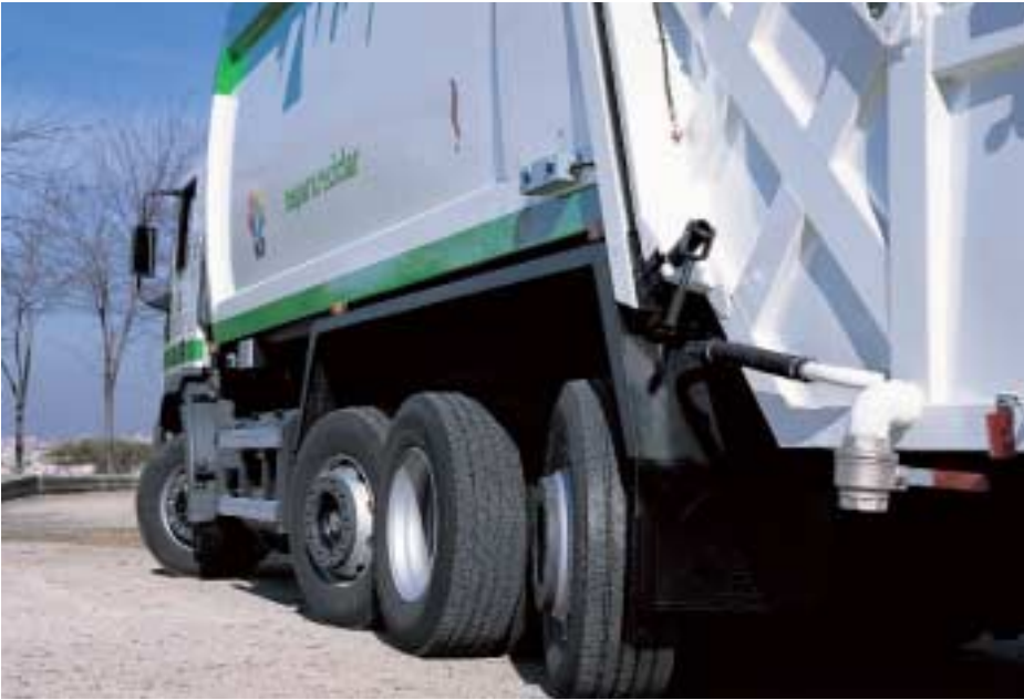
Garbage truck with three drive axles
