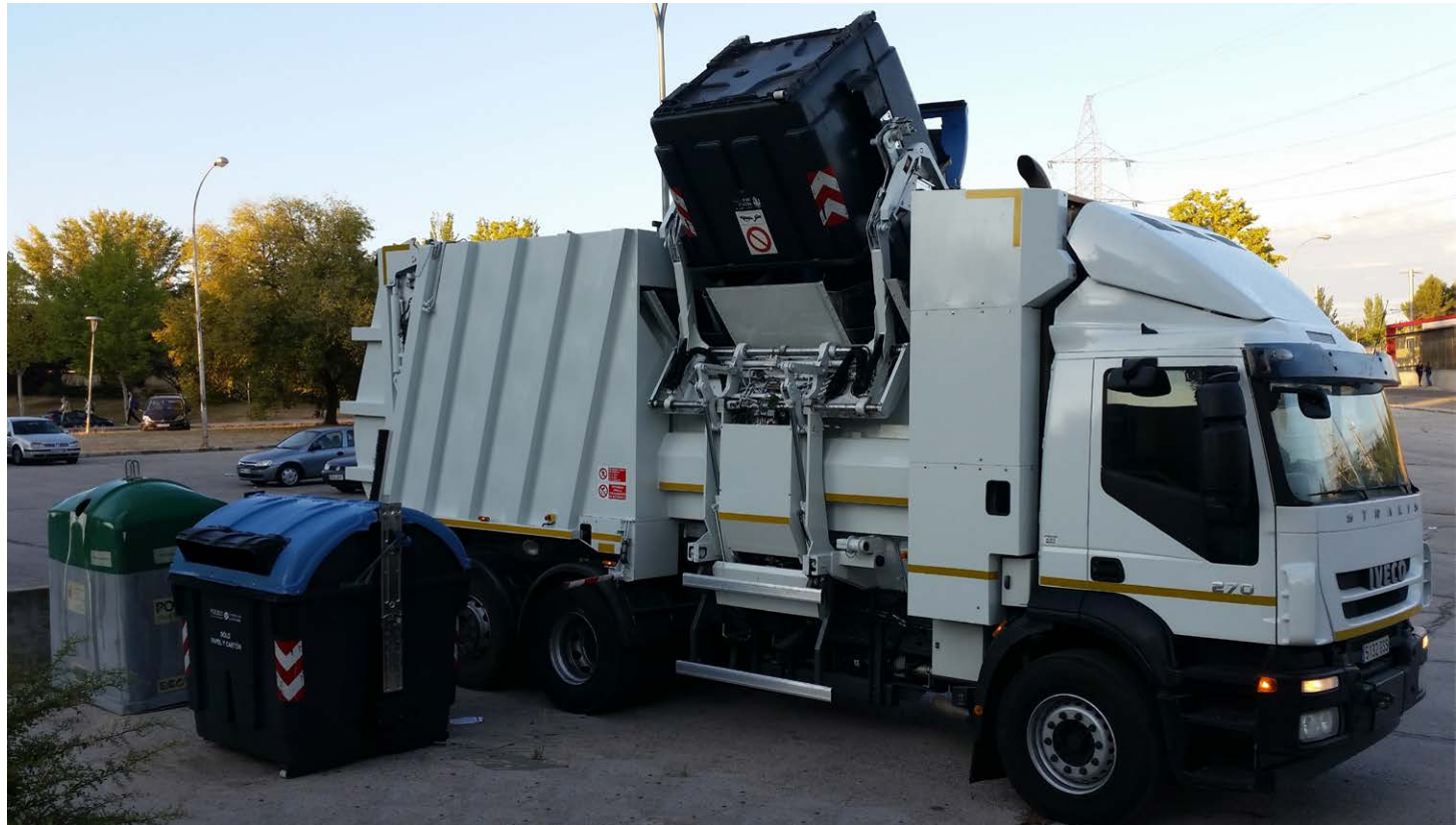
Ultra-capacitor vehicle for MSW.
