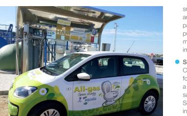
Volkswagen with which Aqualia is testing the biogas produced in the El Torno treatment plant (Chiclana, Cádiz) from the All-gas innovation project.
